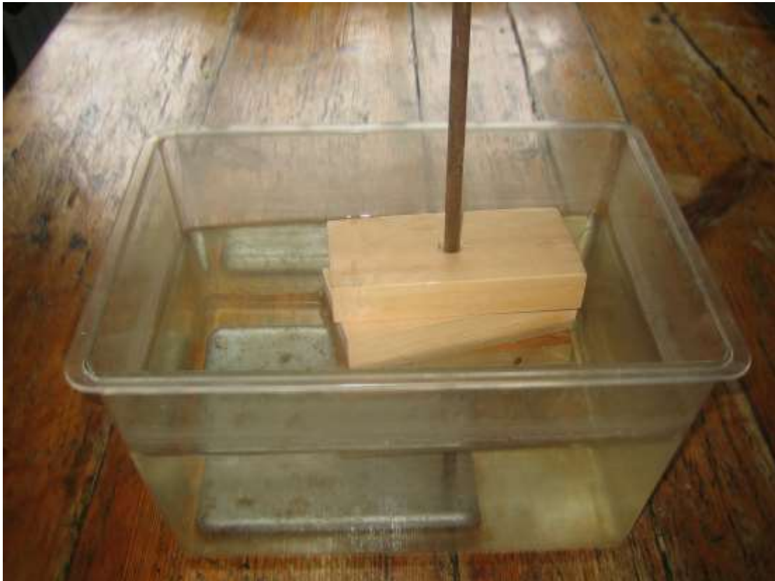
Isostasy; wooden blocks floating in tank
