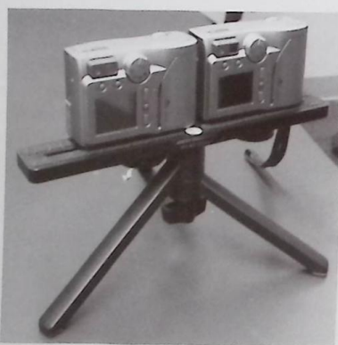
Figure 4. A pair of digital cameras fixed to a frame, for taking stereo photos. This is a useful apparatus, because the separation of the camera lenses can be controlled and measured accurately.
