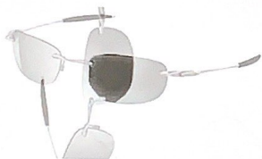
Figure 3. Two polarising sunglasses placed at right angles to each other. Polarised light from the first lens is not allowed through the second lens at right angles.
