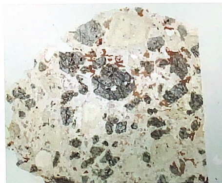
Figure 5. Mineral slide photographed using a standard 35 mm digital six megapixel camera, hand held. Even better results could be obtained using a tripod and a high f stop number.
