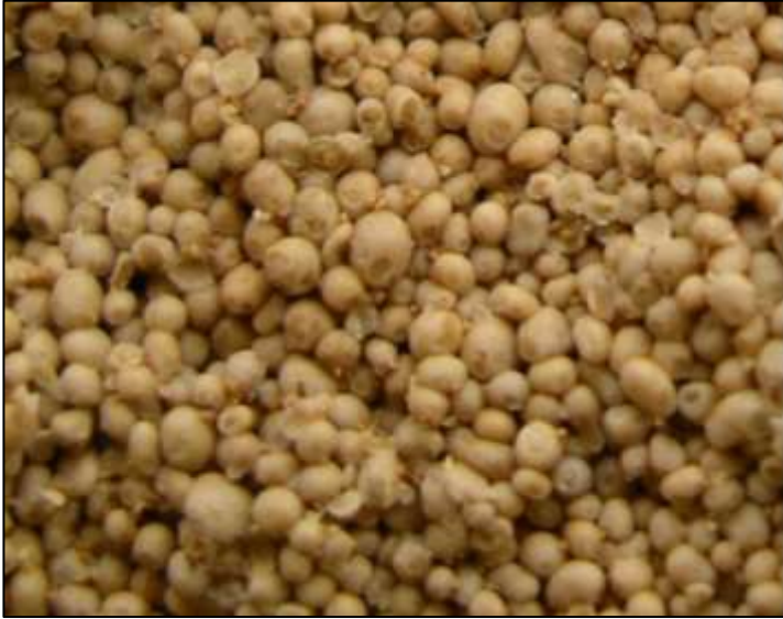
Figure 4: Fracture surface of oolitic limestone from the Lincolnshire Limestone at Ketton. Diameter of ooids \sim 0.5\text{mm}
