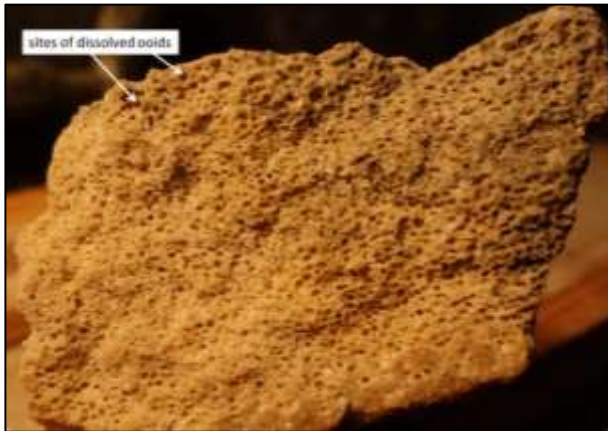
Figure 16: Hand specimen (50mm) of Magnesian Limestone from Sunderland. The ooids have dissolved leaving a high degree of porosity.
