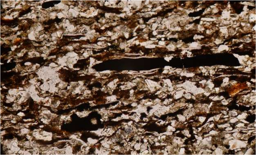
Figure 20: Photomicrograph (ppl) of a Westphalian sandstone showing mica flakes (dark brown/black). 2mm field of view.
