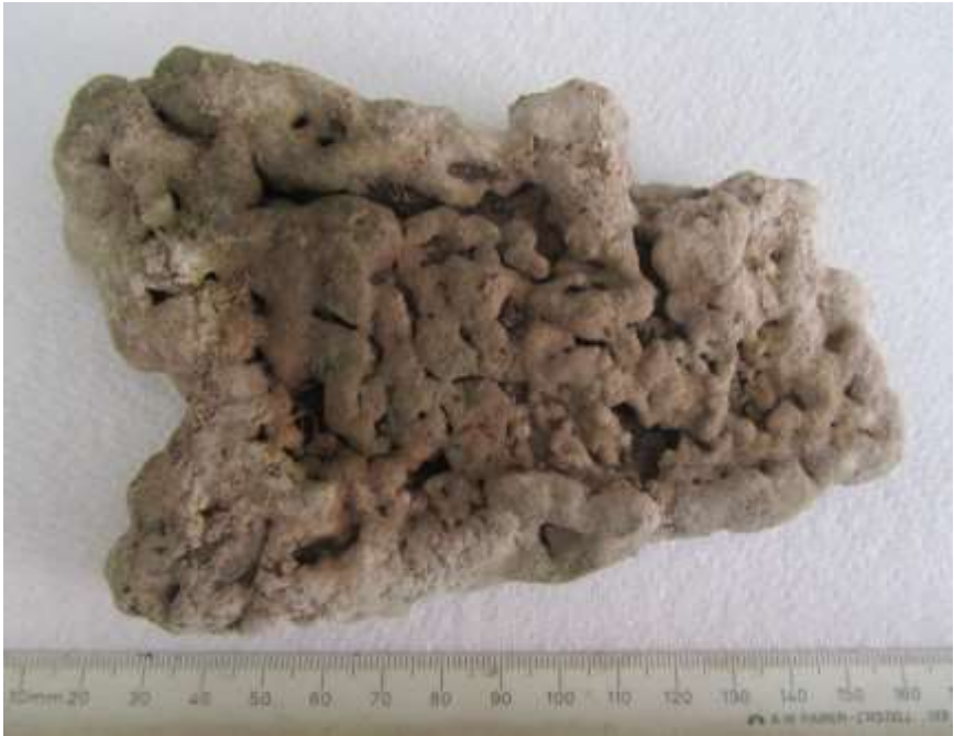
Figure 9: A large piece of bark, ~ 15 cm in length, entirely covered by a heavy coating of tufa. This specimen was recovered from the most southerly channel in Shotwick Dale where tufa is deposited.
